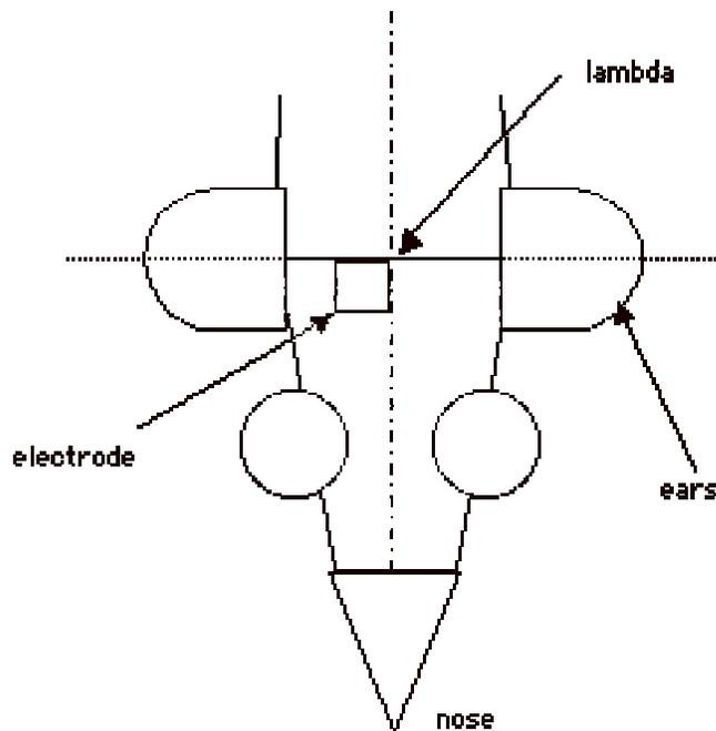
**Figure 1:** The electrode array is placed as shown in the diagram at the corner of lambda. Embedded within the 4 mm by 5 mm Delrin coating, are 12 stainless steel electrodes spaced 1 mm apart.
